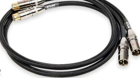
Silver betters both copper and gold for electrical conductivity, as reflected in the Mavros's 70mohm/m loop resistance, slightly higher than the Asimi's 56mohm. Otherwise, the Mavros Ultra offers a lower capacitance and, usefully, lower inductance at 82pF/m (86pF, Asimi) and 0.25µH/m (0.45µH), respectively. So the Mavros Ultra remains a fine choice for long runs.
