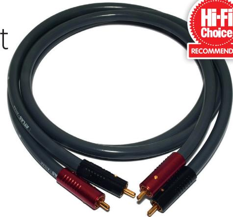
**A COAXIAL CABLE**, the Ailsa Achromatic uses OCC copper for the signal conductor and high-purity OFC copper and copper Mylar foil for the return and shield. A taped microporous PTFE dielectric is employed for the insulation, as in the Asimi and Mavros ranges. The solderless Achromatic plug is connected to the conductors using a cold-welding process.
