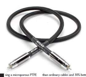
dielectric together with silver-plated copper conductors. The new microporous insulation with a dielectric constant between 1.3 and 1.5 improves on ordinary PTFE and provides up to 85% greater velocity of propagation
